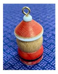
TIP is to apply pen with lathe running at a slow speed otherwise friction will create heat and burn the tips of the pens.
